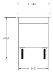
2. Insert the VLC gauge into the opening, making sure it's aligned properly. Then, secure the gauge with the supplied L-brackets and thumb nuts.
