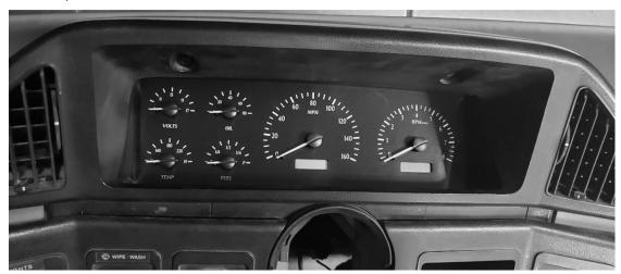
9. Stock 3-Wire alternators may need an additional wiring connection at the gauge cluster connector. You will need to add resistance from the Red/LT GRN wire in the 12<sup>th</sup> pin location to the LT GRN/RED wire in the 11<sup>th</sup> pin location. This will 'excite' the alternator telling it to begin charging. This can be done using the included alternator load harness.
