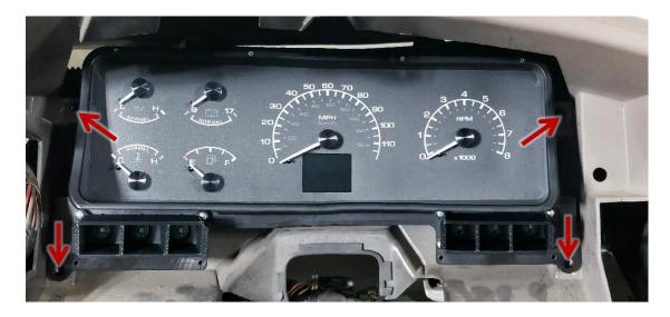
5. Reassemble the dash in reverse order. Refer to the main RTX manual for control box wiring and setup instructions.
