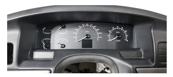
6. Stock 3-Wire alternators may need an additional wiring connection at the gauge cluster connector. You will need to add resistance from the Red/LT GRN wire in the 12<sup>th</sup> pin location to the LT GRN/RED wire in the 11<sup>th</sup> pin location. This will 'excite' the alternator telling it to begin charging. This can be done using the included **Alternator Load Harness**.
