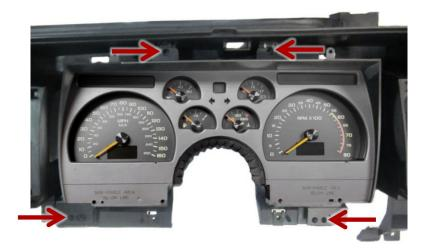
6. Reassemble the dash in reverse order of disassembly using the retained hardware from step one. Refer to the main RTX manual for wiring instructions to complete the system installation.
