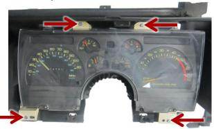
2. The original inner gauge panel and rubber dust seal will be reused; remove the six screws that secure the clear lens and the additional three screws on top that retain the inner gauge panel. Save all hardware for reassembly.
