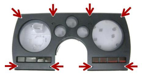
2. Remove the stock gauges, light indicators, and lens from the bezel. The only item to be reused is the original front bezel; the other pieces can be discarded. Now is a good time to clean the bezel.
