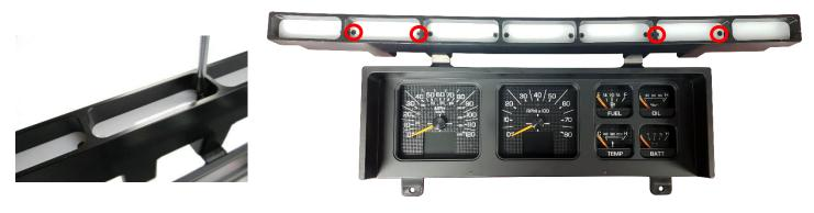
5. Test fit the original gauge housing over the RTX display. If the indicator panel doesn't fit into the housing properly, loosen the eight Philips screws indicated below and adjust as needed. Once adjusted, lightly tighten the Philips screws to prevent further adjustment.
