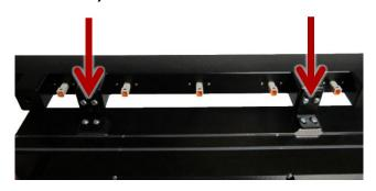
6. Fasten the RTX display into the dash using the original four mounting screws.
