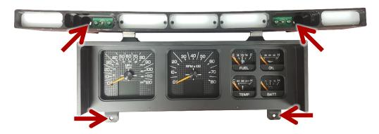
7 Re-install the two white acrylic lenses and four Philips mounting screws.
