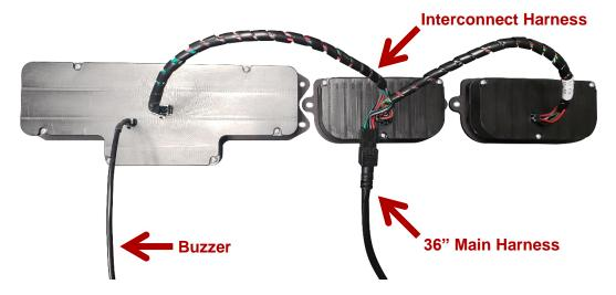
4. Carefully remove the protective lens tape from the front side of the RTX displays. Secure the outer bezel back onto the dash using the original screws. Refer to the main RTX manual for wiring instructions to complete the system installation.
