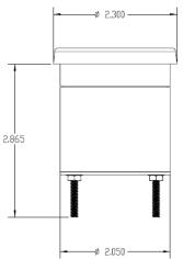
2. Insert the HLC gauge into the opening, making sure it's aligned properly. Then, secure the gauge with the supplied L-brackets and thumb nuts.
