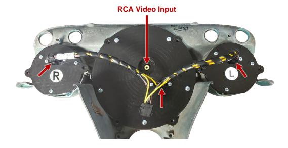
5. Connect the provided **Main Harness** to the interconnect harness. Carefully route the other end of the harness to the control box mounting location.
