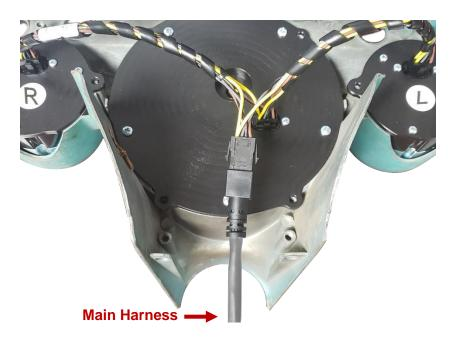
6. Re-install the cluster into the vehicle using the retained factory hardware. Refer to the main GRFX manual for wiring instructions to complete the installation.
