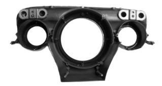
2. Install the new GRFX system using the eight included **8-32 x 3/8" Screws** and **Lock Washers**. Viewing from the back side, mount the gauge labelled "R" on the left, and "L" on the right.
