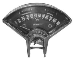
2. Remove the six screws holding the gauges to the bezel from the back of the system, so the stock gauges, separator plate, and lens can be removed.
