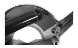
5. Next, cut the supplied **Foam Tape** into four small strips, approximately 1" long. Install these four foam blocks into the bezel to help prevent any potential rattling. The foam should sit down in the bezel and adhere to the outer edge, sticking up about 1/8" to compress against the lens once the system is installed.
