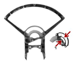
4. If you have a bezel for an automatic transmission, attach the provided **Block-Out Panel** with silicone or hot glue; the stock gear position indicator will not fit with the GRFX system. A separate GSS gear position sensor can be purchased from Dakota Digital that will allow the gear position to appear directly on the GRFX system display.
