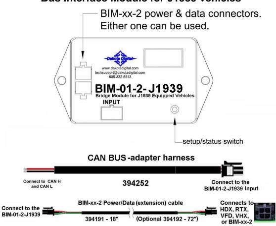
This Bus Interface Module is designed to read engine information from the J1939 bus. The module is connected to the J1939 Bus through CAN bus-adapter harness to the CANH (RED WIRE) and CANL (BLACK WIRE) on the main harness.
