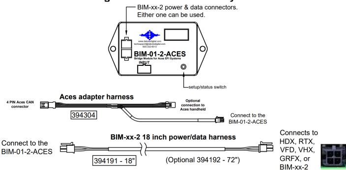
This Bus Interface Module is designed to read engine information from the Aces bus. The module is connected to the Aces CAN bus through the 394304 CAN bus adapter harness.
