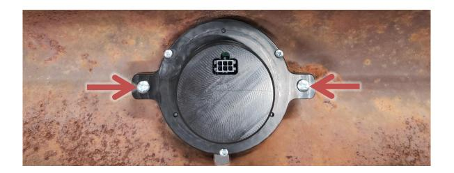
3. Connect the provided RLC harness to the clock and carefully route the other end to the RTX control box. Refer to the enclosed clock operation manual to complete the RLC clock setup.
