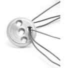
8. Slide the mounting plate over the two studs and tighten it down with the two #6 lock nuts. This will secure the LED assembly into the housing, you are now ready for re-assembly.
